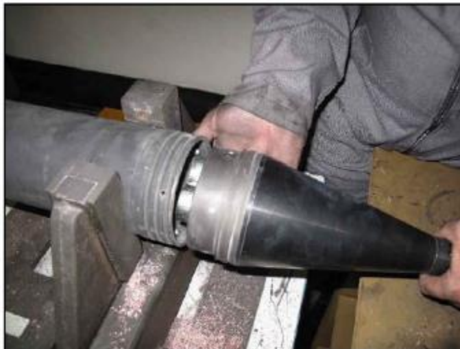
Removal of the M93 tail assembly permits an efficient demolition system
