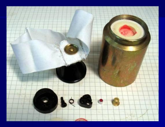
Each submunitions type was broken down into its component parts
