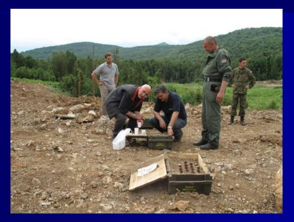
Setting up the burning trial with submunition bodies placed in soil-filled crates
