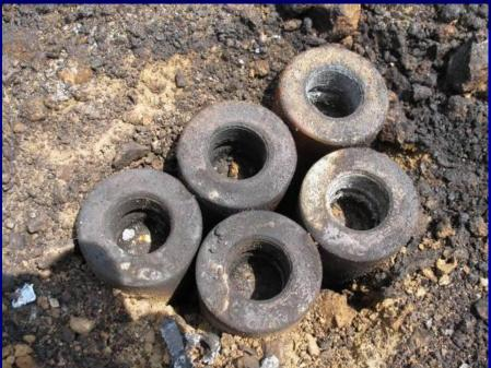
BL-755 bodies, completely burned out. The PTAB-2.5M burn was also successful The trial failed to ignite the explosive in the AO-1SCh and KB-1 bodies. Demolition – better option unless different burning techniques are identified
