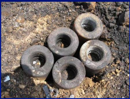
BL-755 bodies, completely burned out. The PTAB-2.5M burn was also successful The trial failed to ignite the explosive in the AO-1SCh and KB-1 bodies Demolition – better option unless different burning technique is identified
