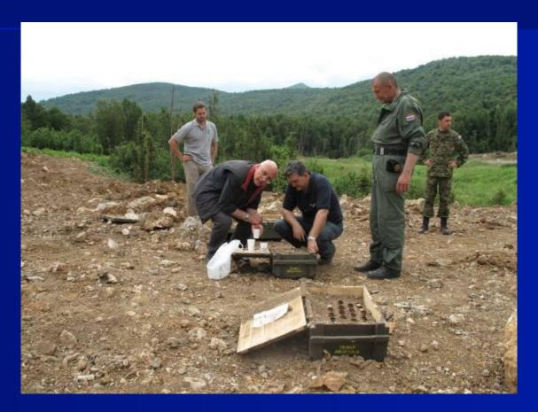
Setting up the burning trial with submunition bodies placed in soil-filled crates
